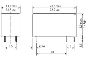
PC board mounting hole layout (BOTTOM VIEW)
