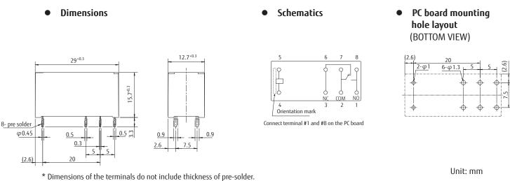
\* Tolerance of PC board mounting hole layout : ±0.1 unless otherwise specified.
