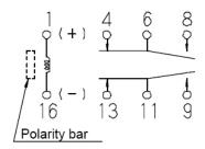
Single Coil Latching type (Bottom view reset position)
