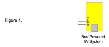
The figure above illustrates a typical USB bus-powered configuration. A USB bus-powered device gets its power from the USB bus.
