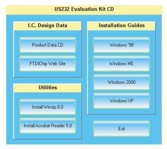
Before plugging the adapter into the PC's USB port, please insert the US232 Driver and Utility CD into the CD drive of the PC. The PC will then display a menu (pictured above) showing the installation guides for the different versions of Windows. These guides are written in HTML and will display on the internet browser of your PC. We recommend that you review the installation guide for your versions of Windows prior to proceeding.
