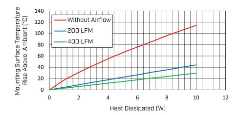
Ths: "hot spot" temperature measured on the heatsink Ta: ambient temperature
