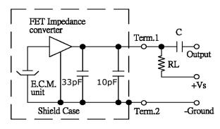
RL =  $2.2 \text{ k}\Omega$ C =  $1 \mu\text{F}$
