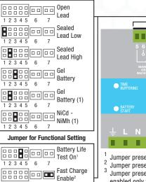
Jumper present: life test enabled. Jumper present: fast test enabled. Jumper present: fast recovery charge enabled only for size 3. Possibility to recharge the battery also when the voltage is close to zero with the maximum power of the device.
