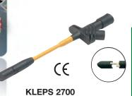
Safety plunger style test probe with spring loaded stainless steel tip, for wires up to 3.5mm, no stripping necessary, 4mm brass socket.
