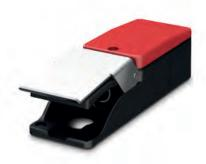
Standard OFF-ON Operation -Lift protective hinged cover up to activate pedal. Push pedal down to change contact state. Release pedal to return to original state. With IP67 Protection Rating (Temporary Submersion).
