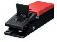
Standard OFF-ON Operation -Push forward in the Anti Trip Pedal Lock to release. Push down pedal to change contact state. Release pedal to return to original state.
