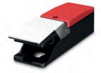
Standard OFF-ON Operation -Lift protective hinged cover up to activate pedal. Push pedal down to change contact state. Release pedal to return to original state. With IP67 Protection Rating (Temporary Submersion).
