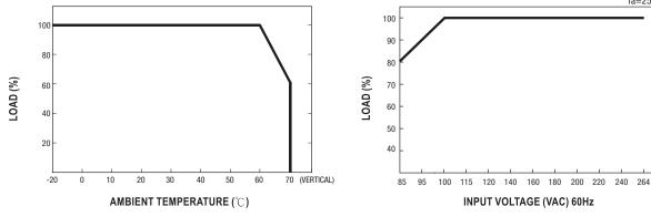
**Output Derating VS Input Voltage**
