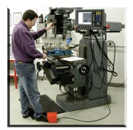
Altech's new low cost foot switch is ideal for any light to medium duty application. The PCFS-3M has an electrical rating of 10A (1/2HP)/125V AC, it can serve as a foot operated on/off switch for a wide range of motor driven and electrical devices.
