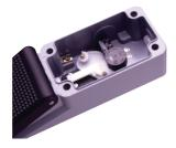
The standard resistance of the potentiometer foot switch is 10k Ohm which provides a proportional signal depending on the position of the foot pedal (Resistances of 100 Ohm to 20k Ohm are also available). Potentiometers are available for the FL and FS Series.
