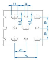
3x4, 4x4 and 6x4" duct does not have middle mounting row of slots
