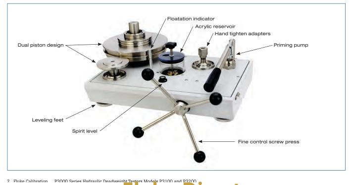
2 Fluke Calibration P3000 Series Hydraulic Deadweight Te
