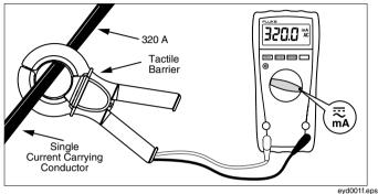
**Figure 1. Current Measurement**
