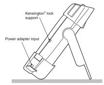
Figure 44. Using the Tilt Stand
