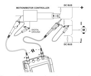
Figure 41. Parasitic capacitance between analog and digital reference
