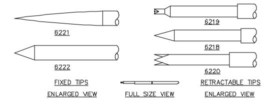
Model 6475 is a set of two each of the following five probes that fit Pomona probes that use the .054Ø test probe tips. Individual replacement probe tips are available in packages of 10.
