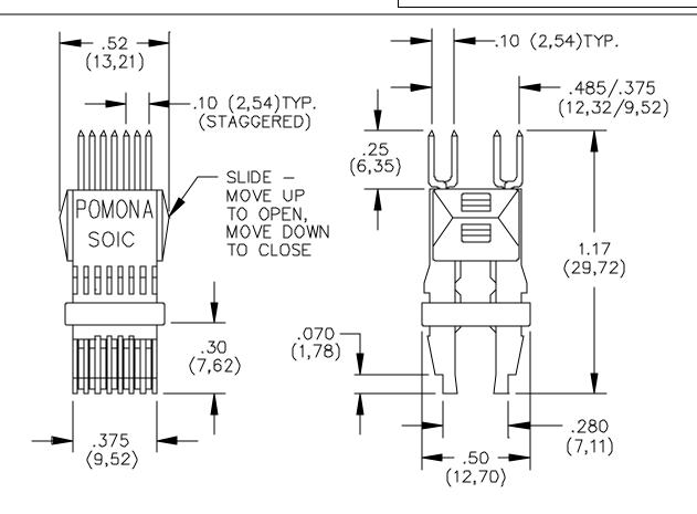
This new test clip is designed for testing .150" (3,81) wide, 14 pin SOIC chips. Model 5413 SOIC Clip® test clip has a positive locking feature that assures a secure connection to all chip leads and provides hands-free testing.
