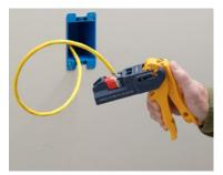
Step 6: Wires will be seated and cut for a solid termination.
