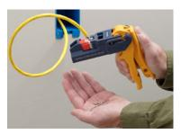
Step 7: Release handle and remove jack from JackRapid tool. Visually verify proper termination.
