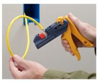
Step 4: Ensure jack is completely and securely inserted in jack holder bed with IDC slots facing the blades.
