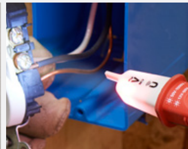
Built-in worklight (NCV-1030, NCV-1040)
