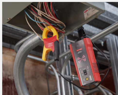
Intuitive transmitter automatically senses whether the system is energized or de-energized
