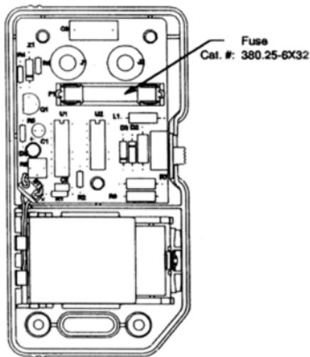
Fig. 10b: X1000 with Front Cover Removed
