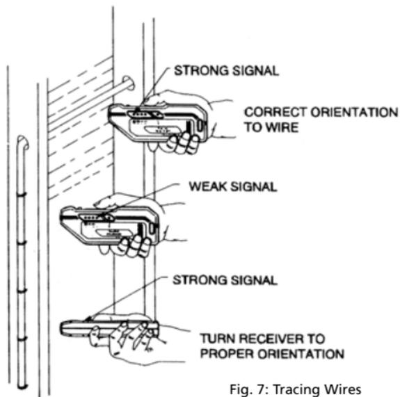
In the "Current Mode", orient the Receiver so that it is perpendicular to the wire.
