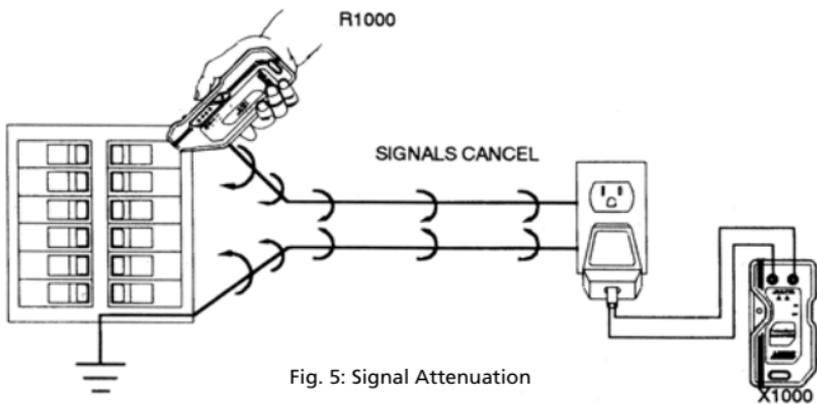
Fig. 5: Signal Attenuation
