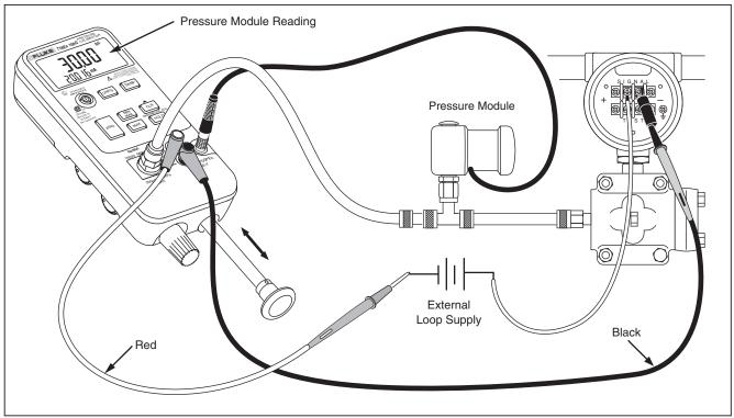
Figure 5. Pressure Module with Internal Pump
