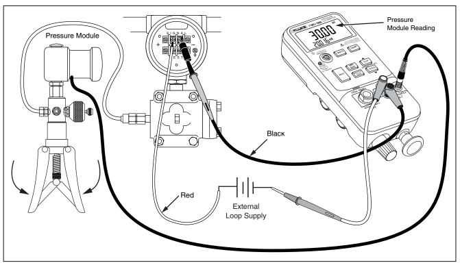
Figure 6. Pressure Module with External Pump
