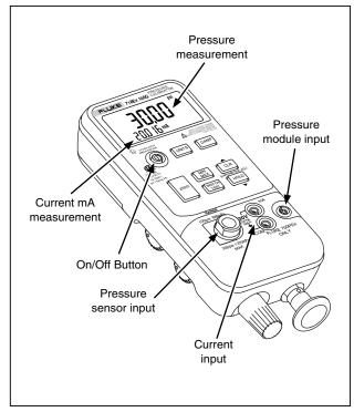
Figure 2. Front Panel Features
