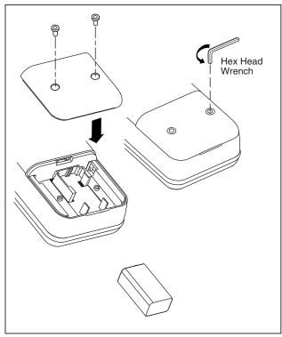
Figure 7. Battery Replacement
