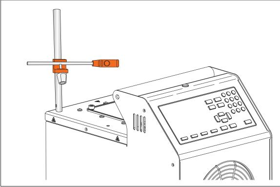
Figure 8. Probe Clamp Accessory
