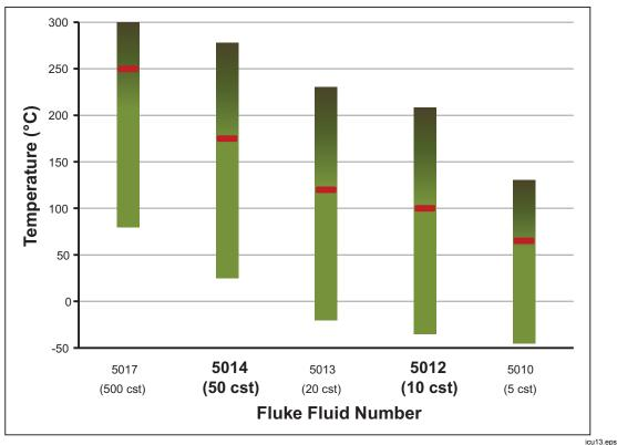
Figure 15. Silicone Fluid Temperature Ranges
