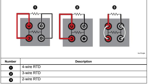
Figure 12. Test RTD Connections
