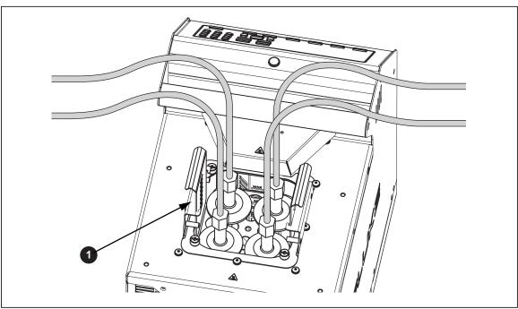
Figure 9. Adjustable Probe Fixture
