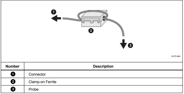
Figure 10. Ferrite Installation
