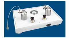
testers providing a rateless liquid-to gas separation. Driven by a pneumatic pressure source (nitrogen bottle) and controlled by needle valves, high pressure gas is balanced against the liquid in a hydraulic deadweight tester through a series of fluid traps.
