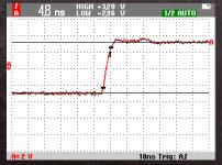
5GS/s sampling or 200 ps sample resolution provides the detail needed to inspect signal edge dV/dt or signs of destructive reflections.
