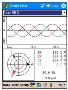
View measurements real-time with wireless PDA interface.
