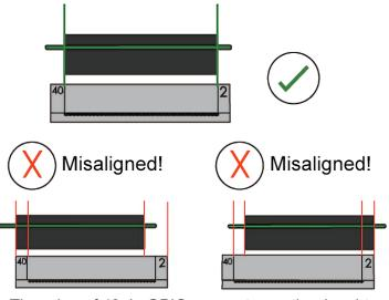
The edge of 40pin GPIO connector on the daughter board should align with the alignment mark of grey female socket, the mark "40", "2"&"1" should align with the pin# of GPIO connector.
