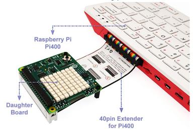
2.Align the pin# of daughter board with the mark on grey 40pin connector, make sure Pin#-1,2 & 40 on daughter is aligned with the mark-"1,2 & 40 on the grey female connector, insert the daughter board into grey connector.
