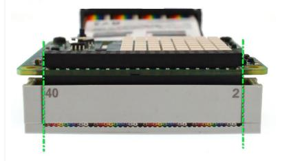
3.Please double check the orientation of daughter board and position of pin#1,2 & 40 base on the below chart before power on Pi400.
