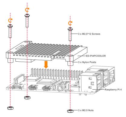
①Place the **ED-Pi4PCOOLER** on the **Raspberry Pi 4** so that the 3 Nylon Post holes align with the 3 mounting holes on the **Raspberry Pi 4**.
