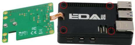
(4)Insert four M2.5\*8+11 studs into the screw holes on **ED-Pi5Case-BB Top Cover** and tighten them clockwise by hand.
