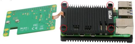
(4) Insert four M2.5\*8+11 studs into the screw holes on **ED-Pi5Case-OB Top Cover** and tighten them clockwise by hand.
