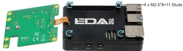
5 Connect the 40-Pin connector to the Raspberry Pi 5.
