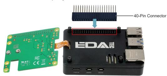
6 Connect the **Raspberry Pi M.2 HAT+** to the **Raspberry Pi 5** via the 40-Pin connector and align the screw holes for the **Raspberry Pi M.2 HAT+** and the 4 studs.
