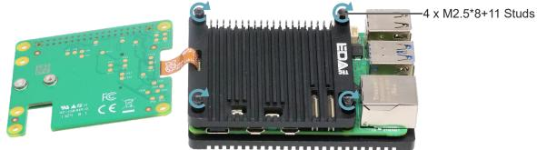
(5) Connect the 40-Pin connector to the **Raspberry Pi 5**.
