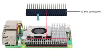
(4) Connect **Raspberry Pi M.2 HAT+** to **Raspberry Pi 5** via 40-Pin connector and plug in the PCIe cable into PCIe port of **Raspberry Pi 5**.
