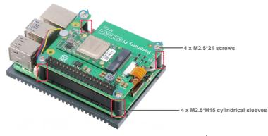
China Phone: +86-18627838895 | Email: sales@edatec.cn / support@edatec.cn EDA Technology Co., LTD ⑦Plug the FPC cable from the **Raspberry Pi Camera Module 3** into the CAM/DISP port on the **Raspberry Pi 5**.
