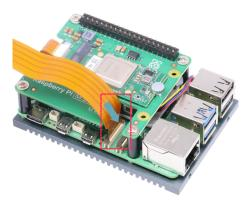
8 Put **ED-Pi5Case-EXT Top Cover** over **ED-Pi5Case-EXT Bottom Cover**, and align the screw holes. Then insert four M2.5\*4 screws and tighten them clockwise using a screwdriver.
