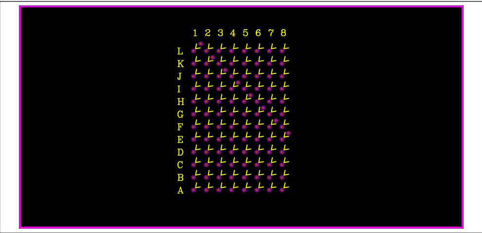
Figure 8: LED Board Component Placement Guide - Top Layer
