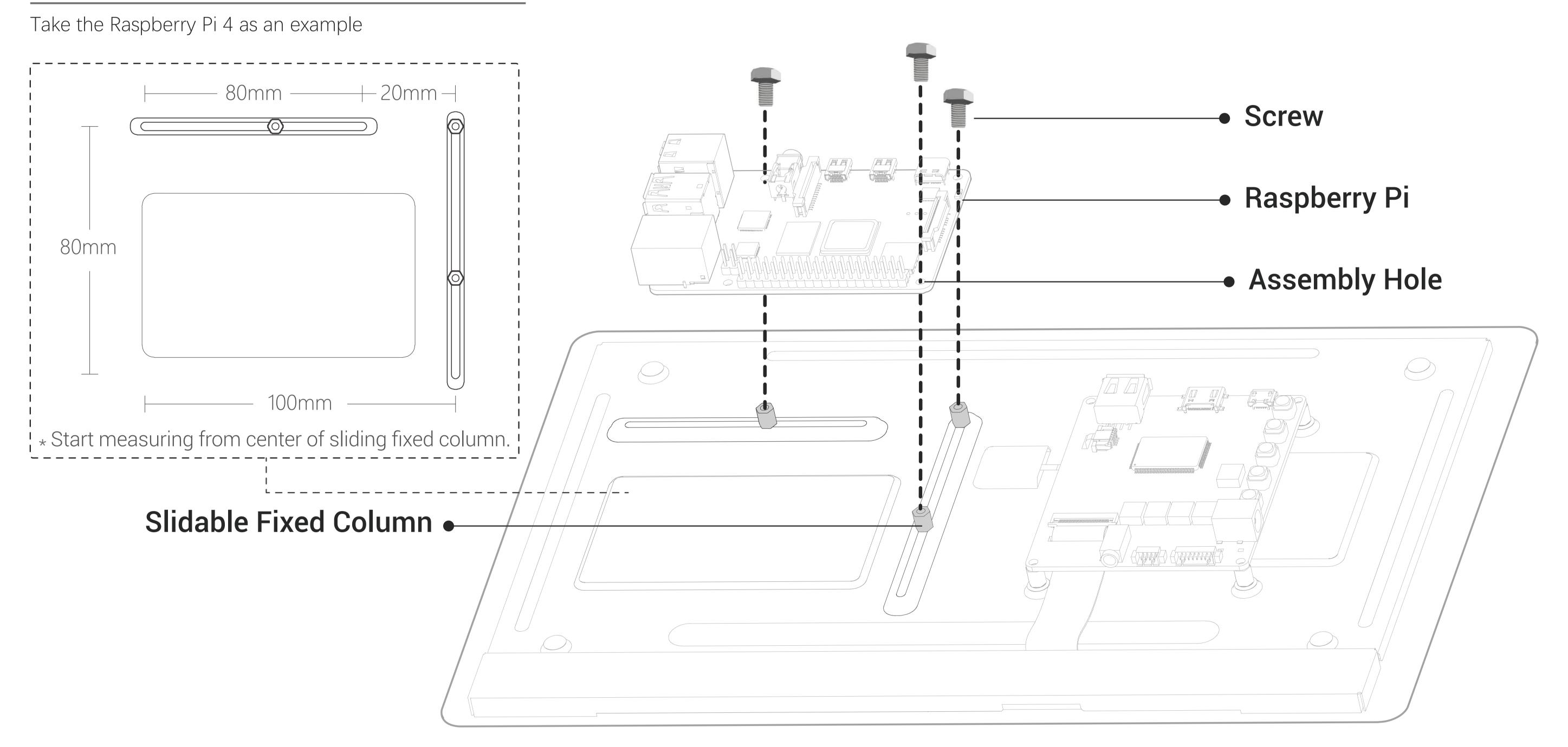
Adjust the sliding retention post to match the Raspberry Pi and attach the screws to the CrowVision sliding retention post through the Raspberry Pi's fixing holes.
