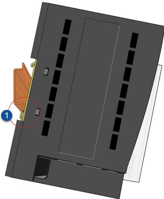
2. Push the bottom part of the module upward, making sure that you feel the clip catch on to the rail, and simultaneously push the
