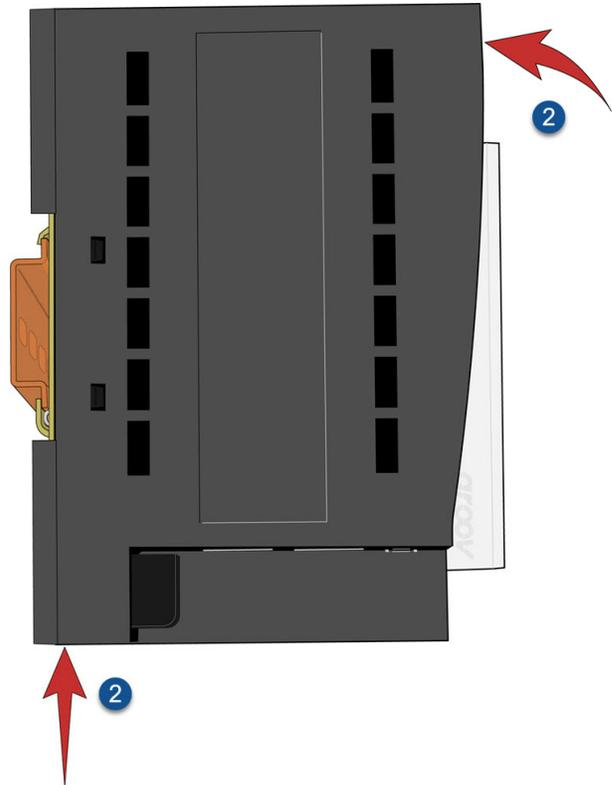
Before you release the module, verify that the top and bottom of the DIN rail adapters have engaged the DIN rail.
