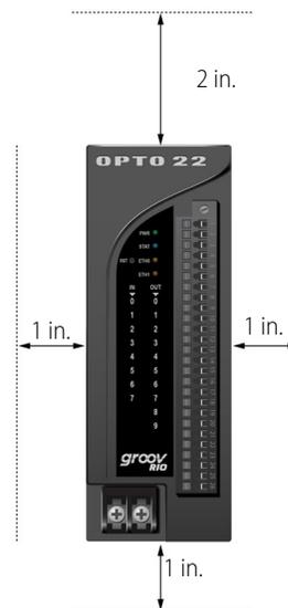
Make sure that there is a minimum of 2 inches clearance on the top, and 1 inch clearance on the bottom, each side, and in front of RIO, after it is mounted. Mount RIO as shown in the diagram: with the Opto 22 logo at the top. Compliance with these guidelines helps ensure that *groov* RIO performs as described in the specifications.
