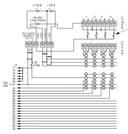
Install 1/8 amp fuse here to use the 24 VDC shared loop source. With fuse installed, shared loop source +24 VDC is available at lower B terminal. Fuses are provided with the AD3 module.
