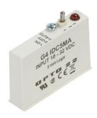
**Opto 22 G4 digital input modules** include the G4IDC5B high-speed module and the G4IDC5MA module with manual-on/manual-off/automatic switch for diagnostic testing.
