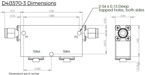
**Connector Configuration** Type of Device PN Suffix PN Example Input / Output N/A Female / Female D4I3570 Single and Dual Junction -1 Male / Female D4I3570-1 Isolator, 2-Port Device -2 Female / Male D4I3570-2 Input / Output -3 Male / Male D4I3570-3
