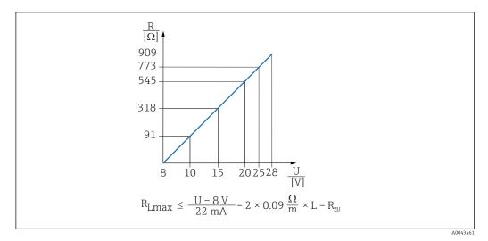
$R_{Lmax}Max$ . load resistance [ $\Omega$ ]
