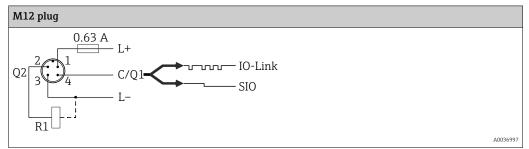
1 x PNP switch output R1 with additional analog output 4 to 20 mA (active)
