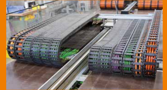
Bend factor test, 76 million strokes at 9.4 x d
