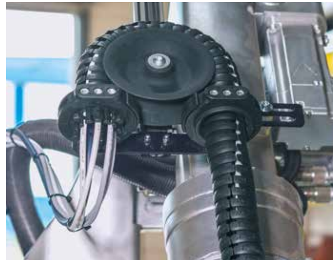
triflex® TR.RSE.40.L or R, cost-effective and lightweight retraction system with deflection roller, for small robots
