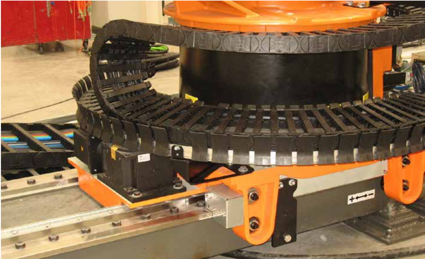
twisterchain application on the robot 7th axis
