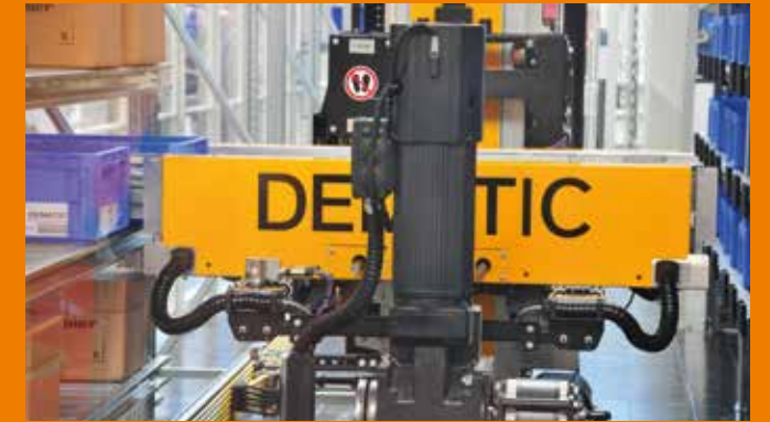
triflex® R in storage and retrieval system
