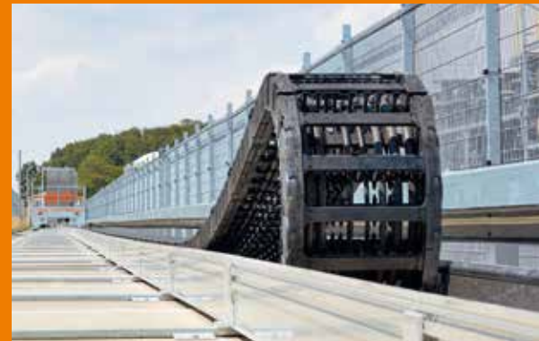
Outdoor test facility for travel lengths of up to 400m
