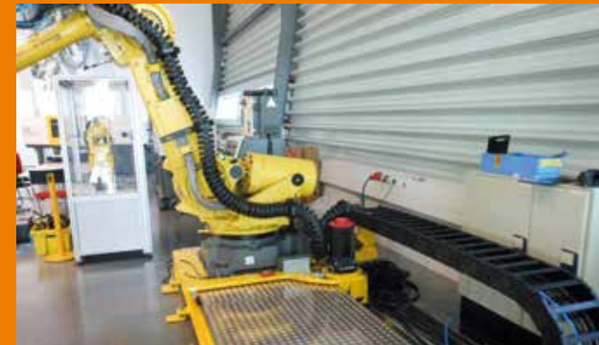
triflex® R on axis 1-6, E4.1 on axis 7 of the robot
