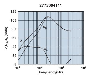
Impedance, reactance, and resistance vs. frequency.
