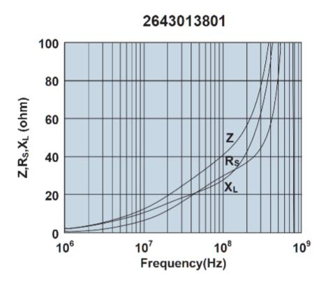
Impedance, reactance, and resistance vs. frequency.
