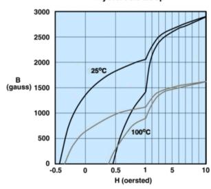
Measured on a 17/10/6mm toroid at 10kHz.
