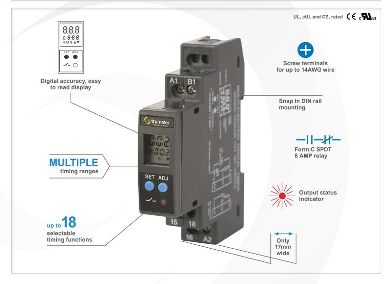
Trumeter's new range of digital time relays offer 8 or 18 operating modes, easily configured on the 3 digit LCD display: a wide range of 0.1s - 999Hr to suit all applications; a clear indication of the relay status via the front panel LED; can accept a wide range of operating voltages for most installations. The keylock feature means settings cannot be tampered with, for 100% reliable operation.
