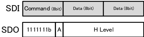
Fig. 18 SPI Write format
