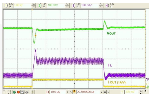
Figure 21. Load Transient, V_{IN}=5\text{ V} , V_{OUT}=2.9\text{ V} , 200-800-200 mA, 100 ns Edge
