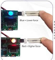
Relative force feedback is displayed on the Prototyping Kit via a blueto-red LED light.
