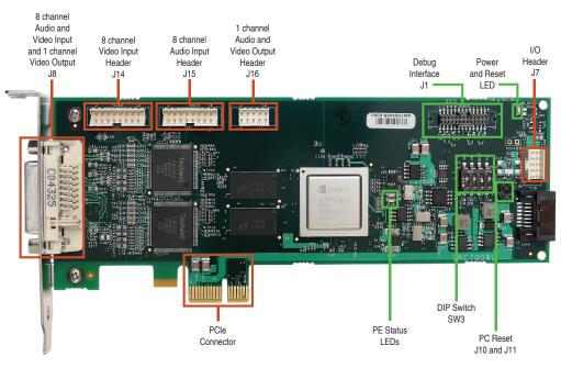
The VRC7008 has a high bandwidth PCIe interface for connectivity with host systems.
