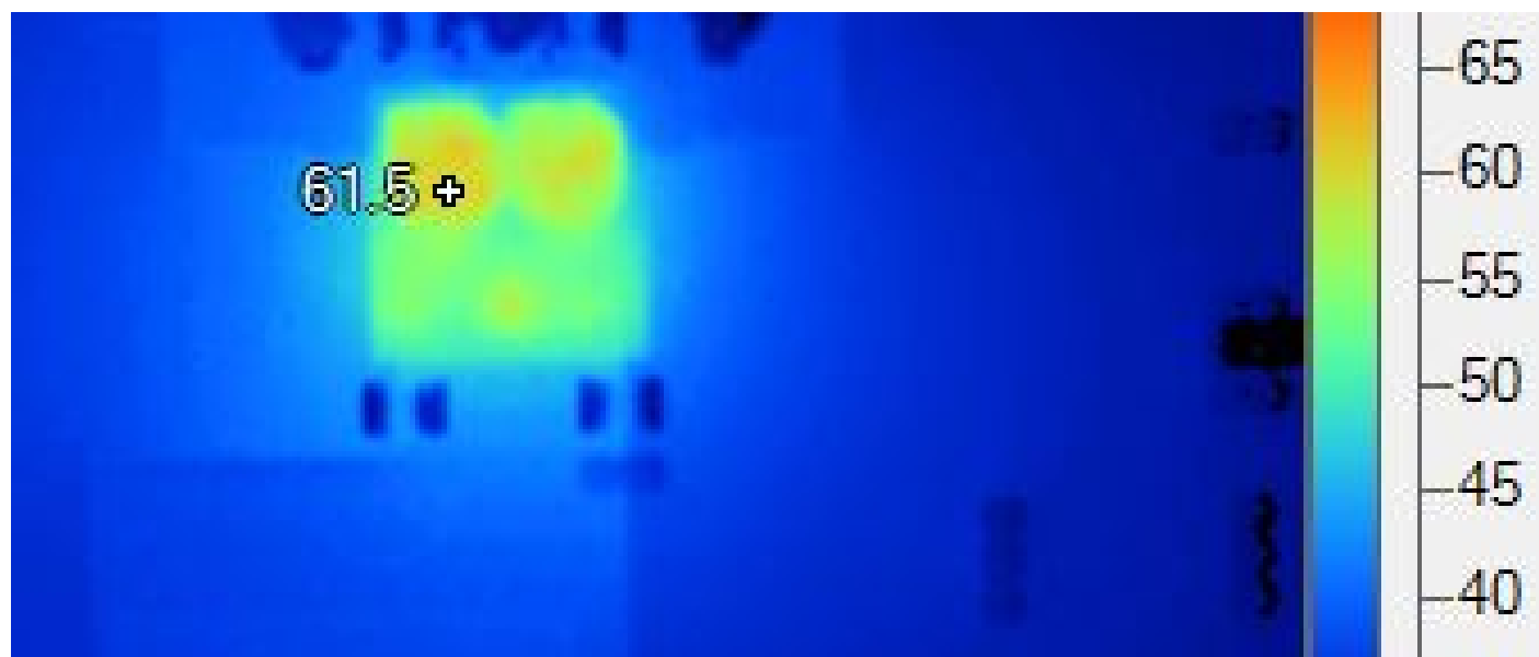
Figure 17: Thermal Image, No Airflow
